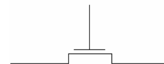
V_G > V_T switch closed
