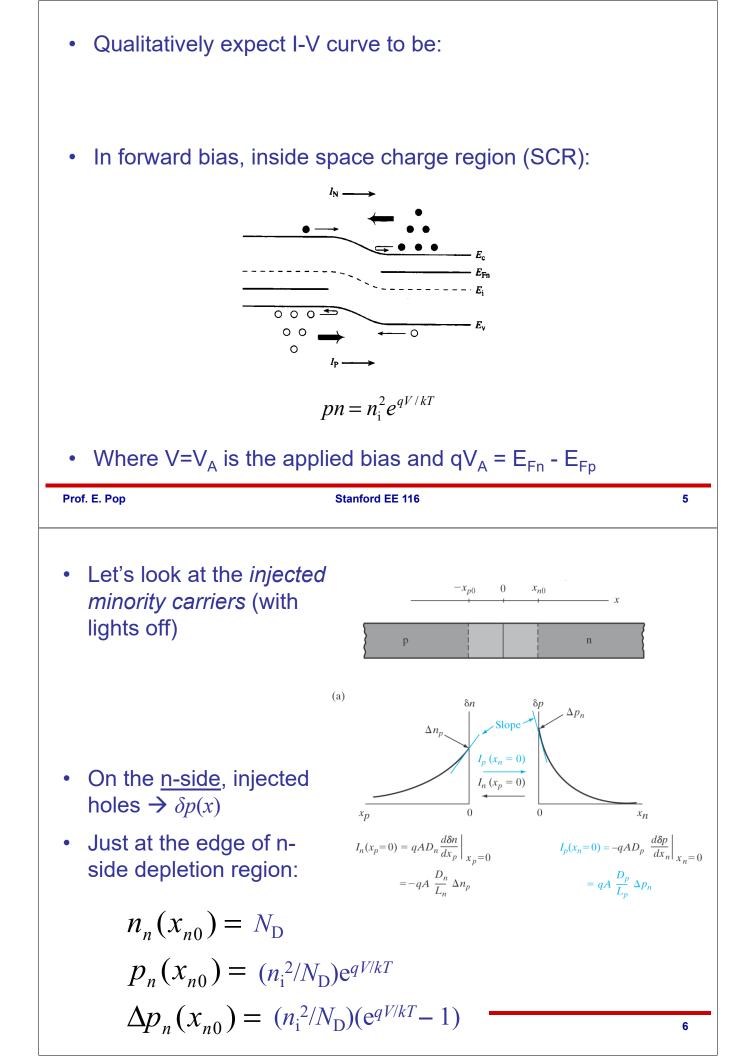
• Excess injected holes diffuse into the n-side:
