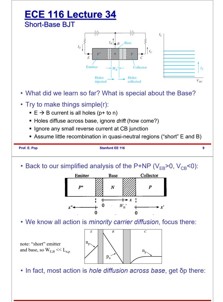
• Now we can *almost* calculate collector (hole) current...
