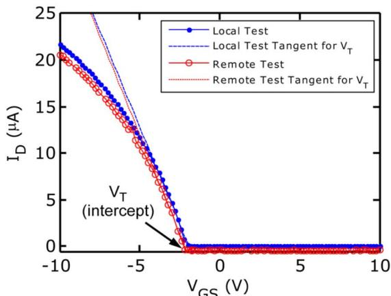
Fig. 6. Comparison of data taken locally in the lab and remotely using the WS shows nearly identical results, validating the WS technique. Here, the drain current ( $I_D$ ) versus the gate voltage ( $V_{GS}$ ) of a p-type MOSFET is measured. The threshold voltage ( $V_T$ ) is extracted using the linear extrapolation method (see text).
