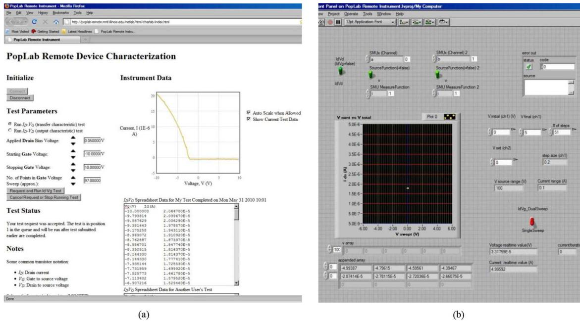
Fig. 3. Screenshots illustrating (a) the Web interface of the remote instrument seen by the user and (b) the LabView VI that runs on the Web server.
