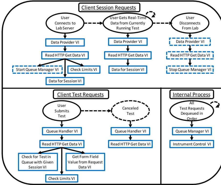
Fig. 4. Diagram of client interaction with LabView server VIs.
