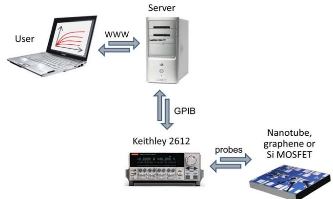
Fig. 1. Schematic of user interaction with remote instrument and test device through the WWW interface.
