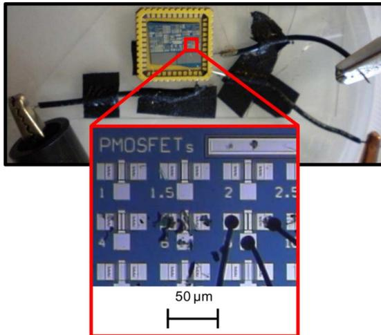
Fig. 5. Photograph and close-up of wirebonded transistors fabricated by undergraduates in the UIUC “Theory and Fabrication of Integrated Circuits” course (ECE 444). In the enlarged image, an individual transistor is wirebonded to the chip carrier, which is then connected to the Keithley 2612 for initial testing of the Remote Lab setup.
