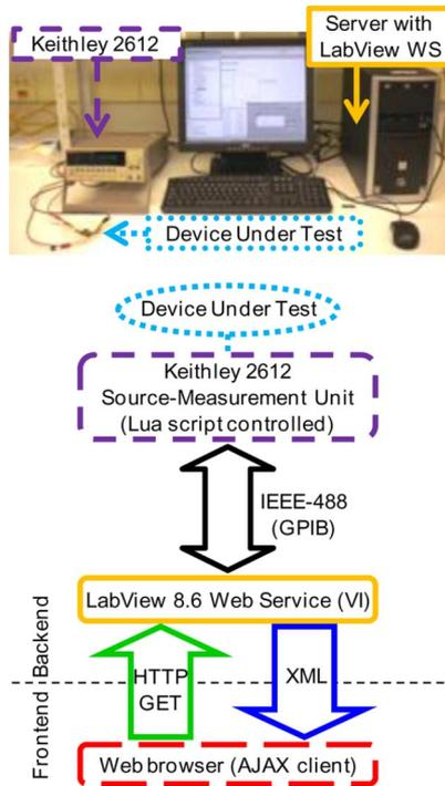
Fig. 2. (Top) Photograph of hardware used for the Remote Lab. (Bottom) Schematic of the remote instrument WS and Web interface architecture.
