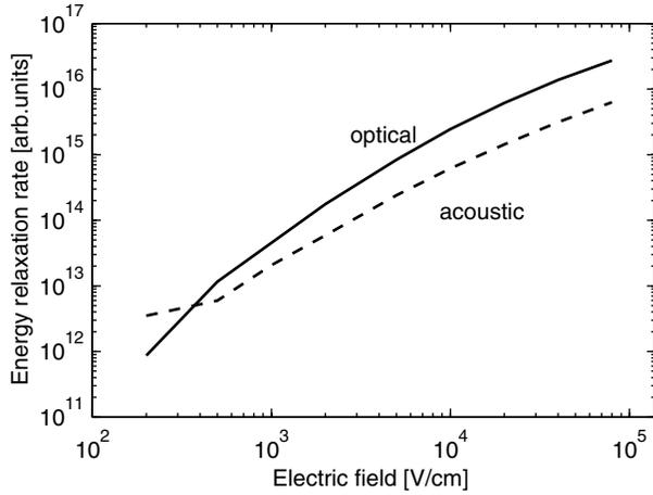
Fig. 4. Energy relaxation rates with optical and acoustic phonons as a function of applied steady-state electric field.
