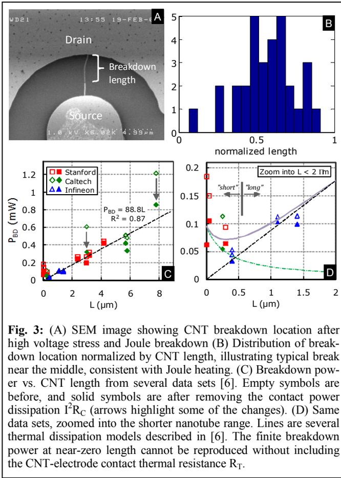
to emerge, showing that the breakdown power of long nanotubes scales linearly with their length (electrode separation), whereas the breakdown of very short nanotubes is almost entirely limited by their contact resistance. The data and models are shown in Figs. 3C and 3D. A minimum in the electrical power required to break single-wall carbon nanotubes is found ( $\sim 0.05$  mW), which may be tailored through careful contact (resistance) engineering.
