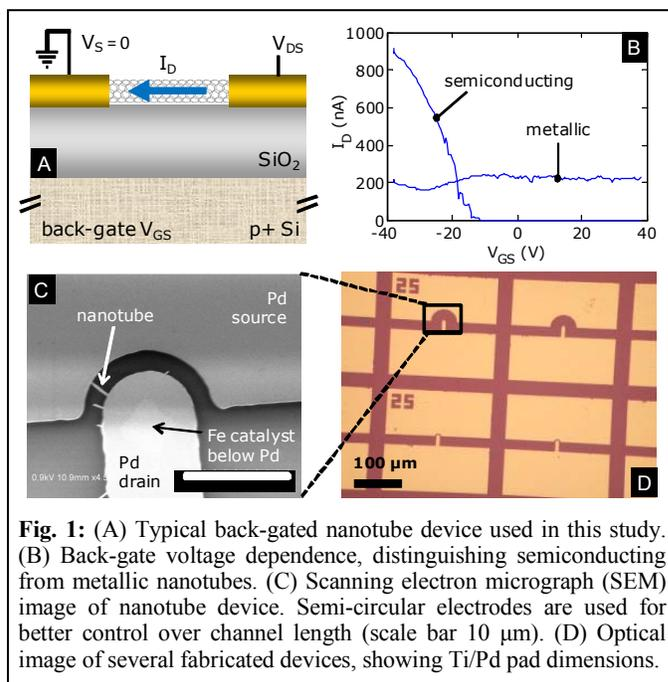
**Fig. 1:** (A) Typical back-gated nanotube device used in this study. (B) Back-gate voltage dependence, distinguishing semiconducting from metallic nanotubes. (C) Scanning electron micrograph (SEM) image of nanotube device. Semi-circular electrodes are used for better control over channel length (scale bar 10 μm). (D) Optical image of several fabricated devices, showing Ti/Pd pad dimensions.
