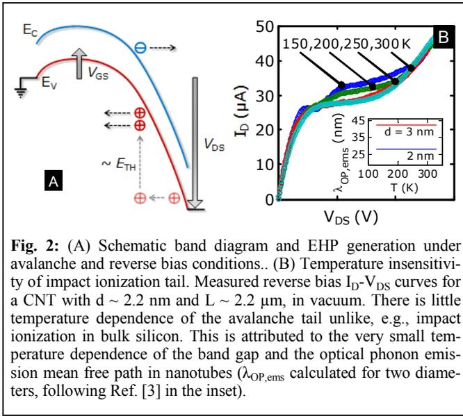
ing in lower longitudinal electric fields and transport by both electrons and holes. In the reverse bias regime, holes are the majority carriers in our CNTs until the avalanche mechanism partially turns on the conduction band (Fig. 2A).
