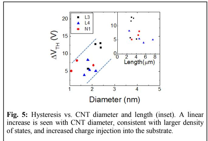
**Fig. 5:** Hysteresis vs. CNT diameter and length (inset). A linear increase is seen with CNT diameter, consistent with larger density of states, and increased charge injection into the substrate.
