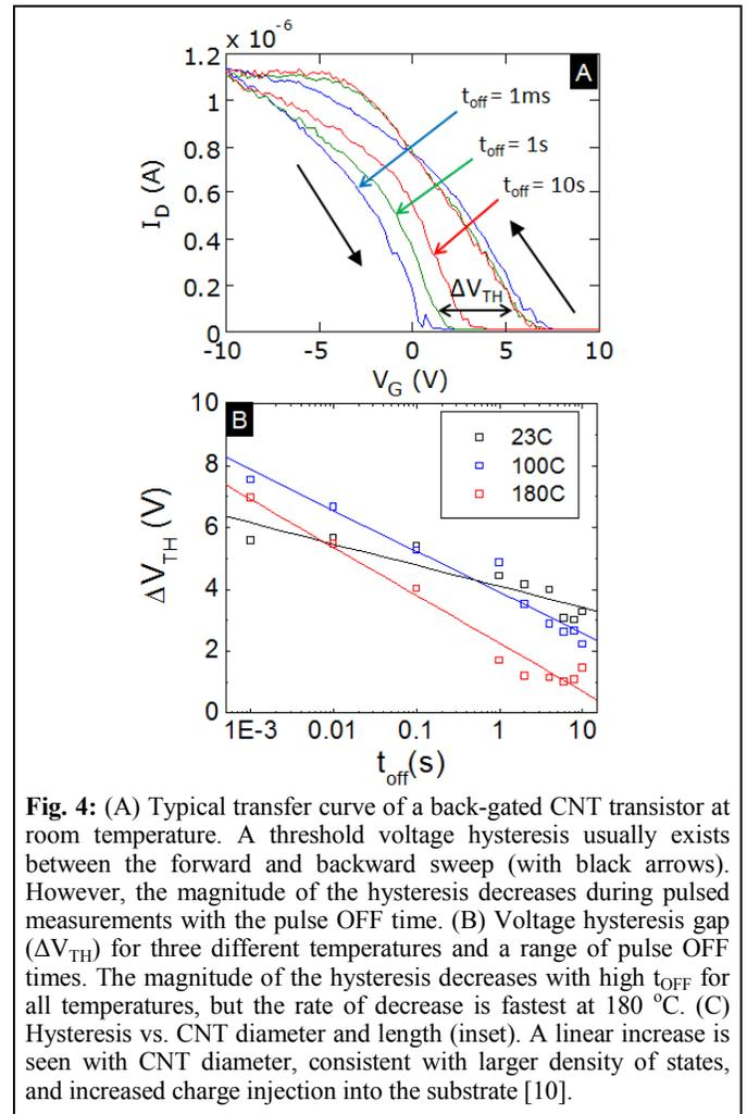
ing to large discrepancies ( $>10x$ ) in reported values as both the forward [1] and backward [9] I-V sweeps have been used. Pulsed measurement techniques have been shown to suppress hysteresis in CNT transfer characteristics [10]. As hysteresis is reduced, both forward and backward sweeps move towards a common, unique central transfer characteristic which reveals the “true” device mobility.
