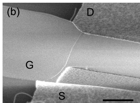
FIG. 1. (Color online) (a) Schematic drawing of our suspended SWNT devices with 10 nm W/20 nm Pt leads. (b) Scanning electron microscopy image of a typical suspended device over  $\sim 2$   $\mu\text{m}$  trench. Scale bar is 1  $\mu\text{m}$ .
