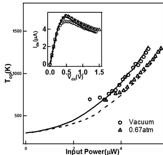
FIG. 3. Calculated  $T_{\text{op}}$  (lines) vs input power for the same device as Fig. 2 at  $T_0 = 300$  K, in vacuum and 0.67 atm argon, respectively. Symbols are  $T_{\text{op}} \approx T_e$  from experimental light emission data and Eq. (2), with the same fitting parameter  $I_0$  as in Fig. 2. The inset shows the experimental  $I$ - $V$  curves (symbols) and fits (lines).
