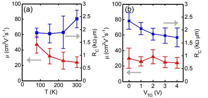
**Fig. 4.** (a) Measured effective mobility ( $\mu$ , red, left axis) and contact resistance ( $R_C$ , blue, right axis) vs. temperature. (b)  $\mu$  (red, left axis) and  $R_C$  (blue, right axis) vs. top-gate voltage ( $V_{TG}$ ). Results obtained from TLM structure shown in Fig. 1f. In-depth analysis of such TLM structures is described in [7].
