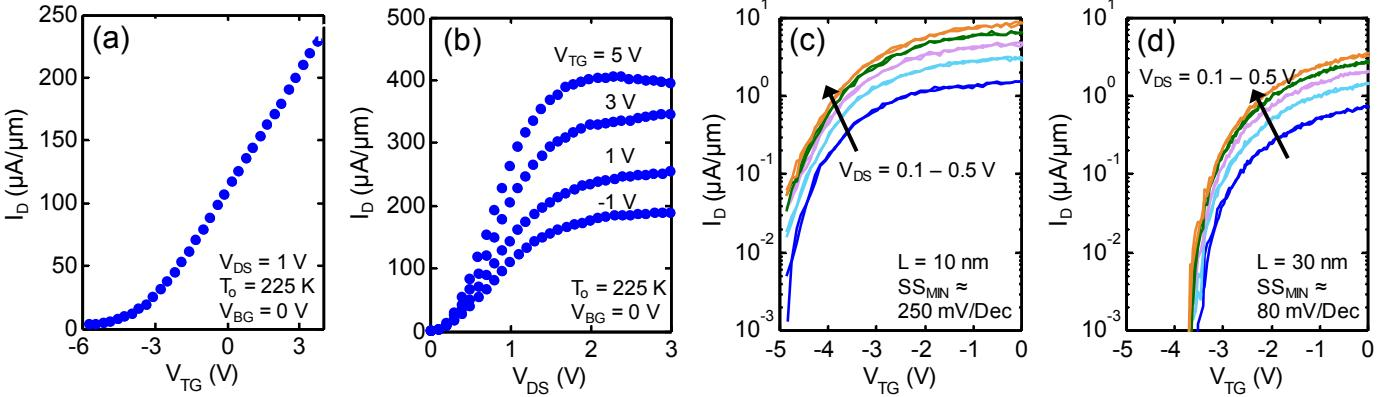
**Fig. 3.** Measurements of short-channel SATFETs. (a)  $I_D$  vs.  $V_{TG}$  and (b)  $I_D$  vs.  $V_{DS}$  at  $T_0 = 225 \text{ K}$  for SATFET with  $L = 10 \text{ nm}$ . (c) Sub-threshold behavior at  $T_0 = 300 \text{ K}$  for SATFET with  $L = 10 \text{ nm}$ , and (d) with  $L = 30 \text{ nm}$ .
